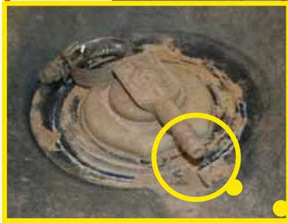
If a vehicle rolls over, you don't want fuel spilling out of the fuel tank. However, you do want air to be able to move in and out of the tank as barometric pressure changes, fuel is added, used, or expands with temperature changes.
