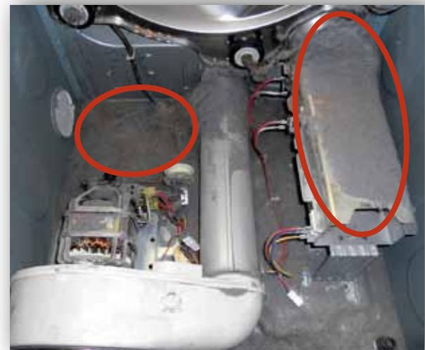
Note the collection of lint inside the cabinet even though the lint trap is cleaned after every cycle! Some manufacturers recommend annual cleaning of the entire appliance by a qualified service technician. Needless to say, I cleaned this dryer out. Even with all the protective devices in the world (and this dryer has several), such a load of lint is not good for operation of the dryer.
